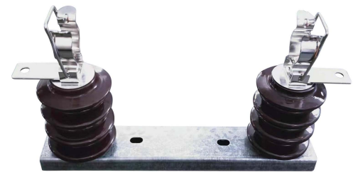
HV Fuse Base (Holder) 3.6/7.2kV for Fuse Link 125A 3.6/7.2kV 63kA Ø76x292 mm
